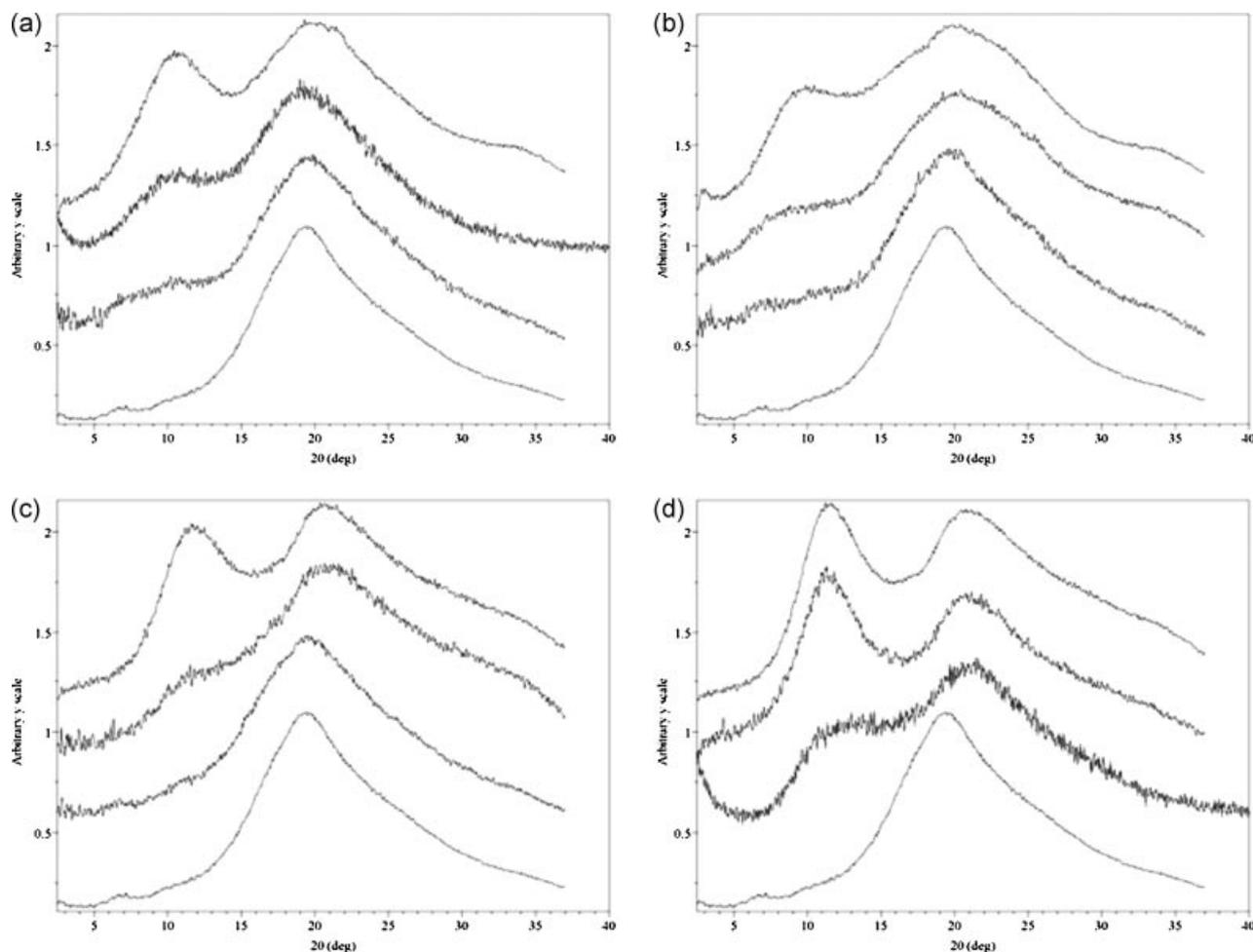
**Figure 3.** Overlay of XRPD patterns for ITZ/polymer dispersions; (a): HPMC-AS, (b): HPMC-P, (c): PVP K-12, and (d): PVP K-90. For each panel (top to bottom); polymer only, 1:2 and 2:1 (w/w) ITZ/polymer, and X-ray amorphous ITZ prepared by melt-quench.
