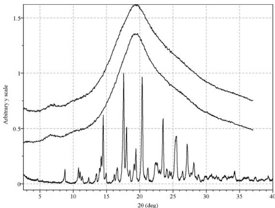
**Figure 2.** Overlay of XRPD patterns (top to bottom); melt-quench cooled ITZ, cryo-ground ITZ at 30 min, and crystalline ITZ as received.
