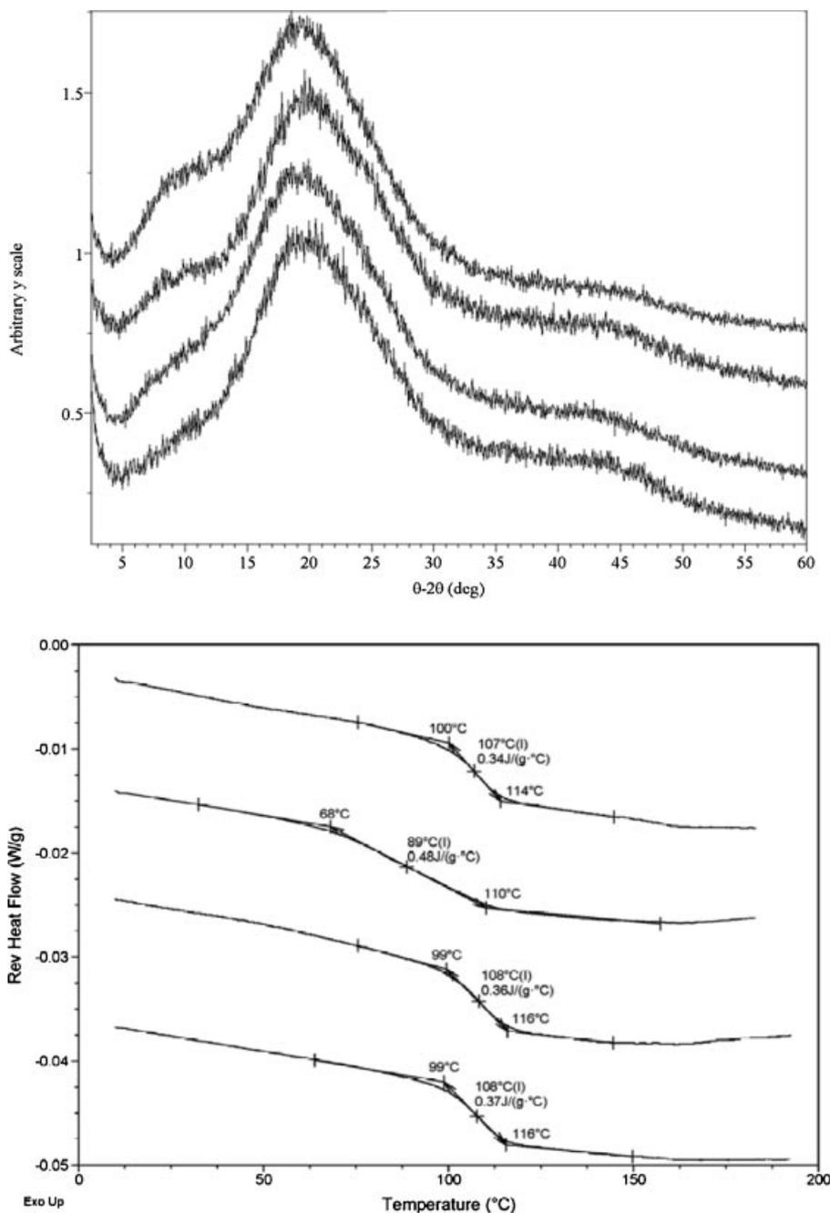
**Figure 4.** Overlay of XRPD patterns (top panel) and reversing heat flow signal by modulated DSC (bottom panel) for 1:2 (w/w) ITZ/HPMC-P samples, from top to bottom: screening (50 mg scale), rotovap-spray (3 g scale), spray dried (200 g scale), and spray dried (1 kg scale).
