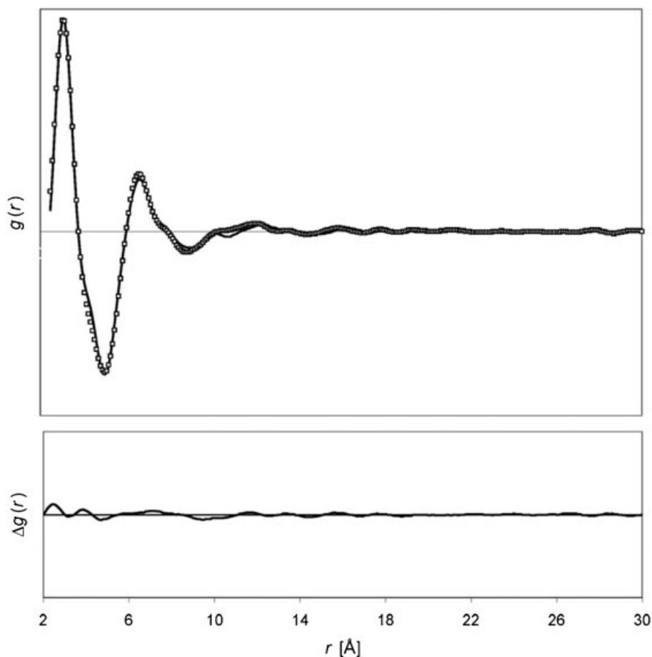
**Figure 5.** Computational analysis of 1:2 (w/w) ITZ/HPMC-P amorphous solid dispersion by PDF method. The PDF acquired from measured data (bold line) is described by the PDF calculated from the individual components (squares), suggesting the sample is a phase-separated mixture.
